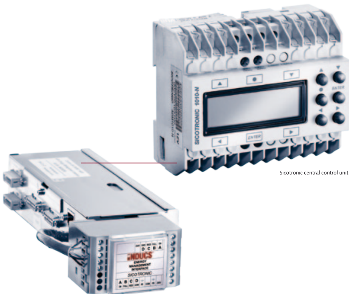
INDUCS control unit with Energy Management Interface
